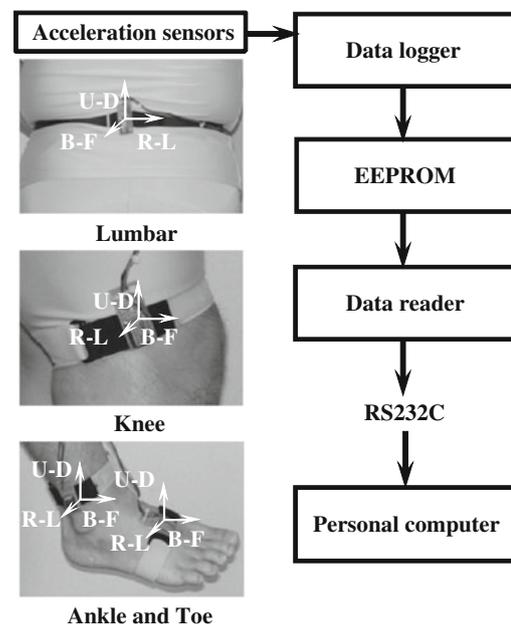
**Fig. 1** Representation of the measuring system for leg motions. EEPROM Electrically erasable and programmable read-only memory, B–F back–front, R–L right–left, U–D up–down
